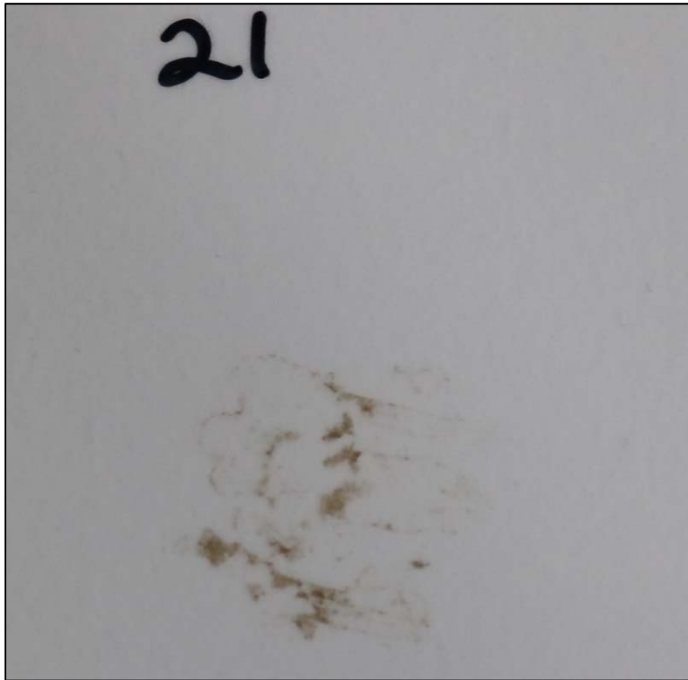
Chemical Spot Test #21, Furfural, Rating 2, Staining
