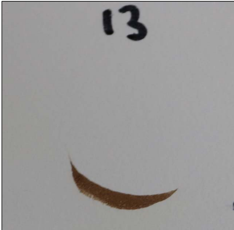
Chemical spot test #13, Chromic Acid (60%), Rating 2, Staining
