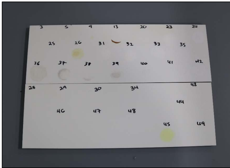
Chemical Spot Test Non-volatile after Exposure, White Sample
