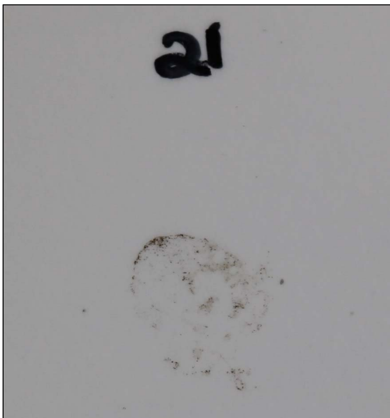
Chemical spot test #21, Furfural, Rating 2, Staining
