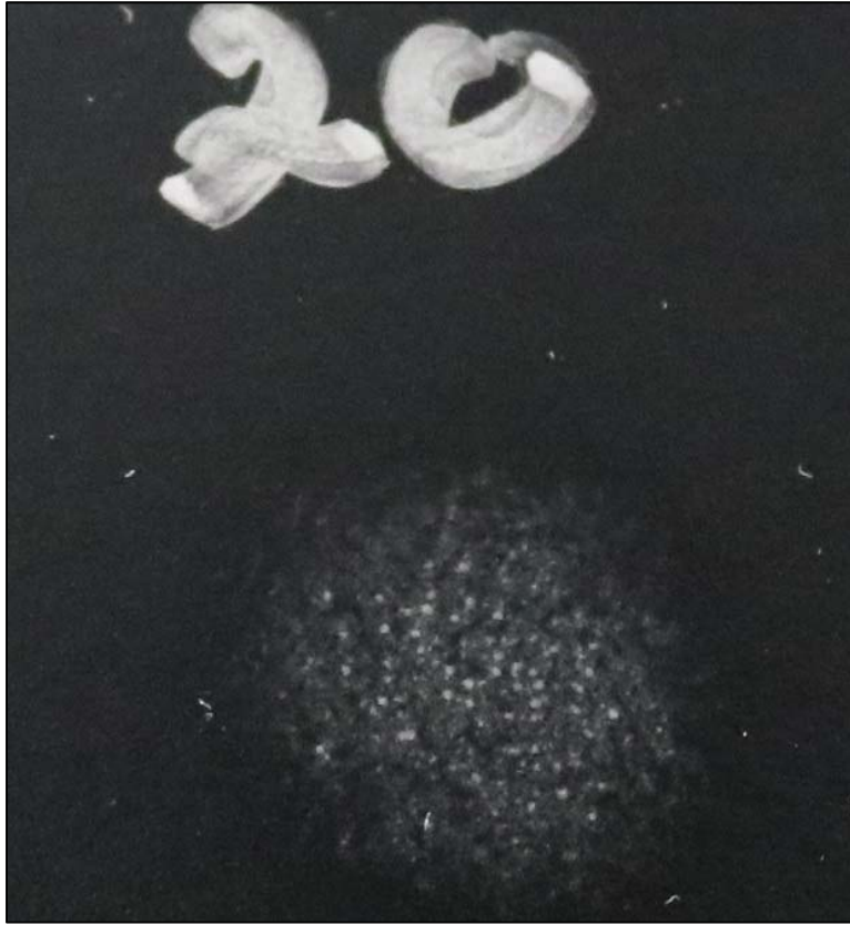
Chemical spot test #20, Formic Acid (90%), Rating 2, Gloss change
