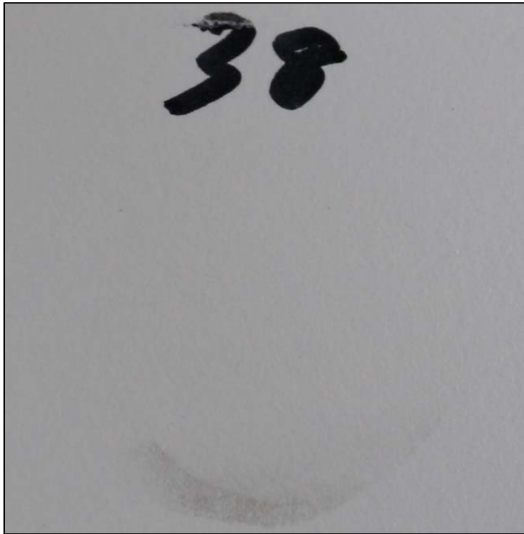
Chemical spot test #38, Sodium Hydroxide (20%), Rating 2, Staining, color change
