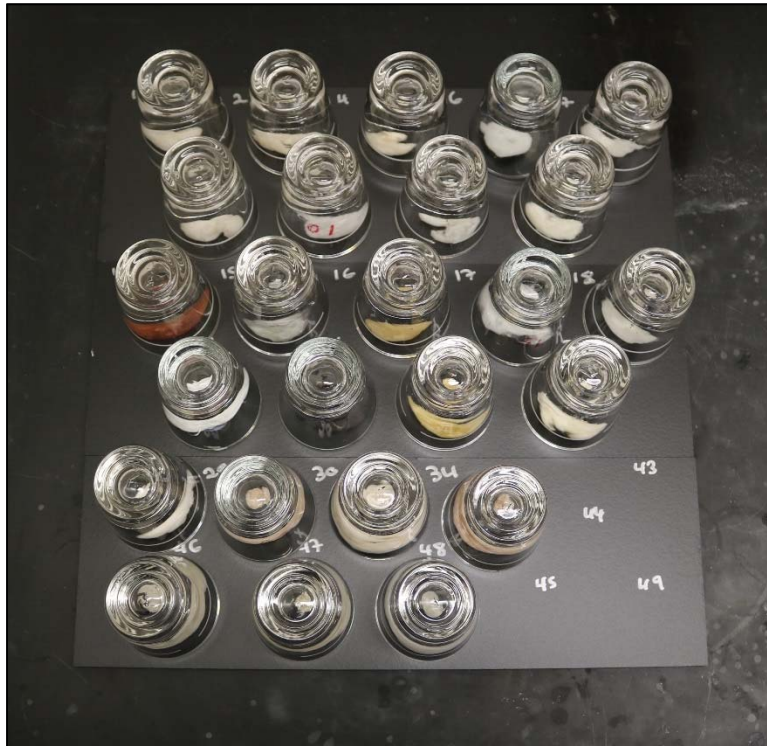
Representative Chemical Spot Test Volatile Chemical Set-up
