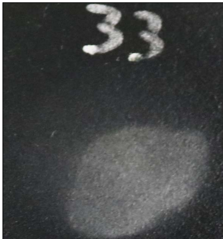
Chemical spot test #33, Nitric Acid (70%), Rating 2, Gloss change
