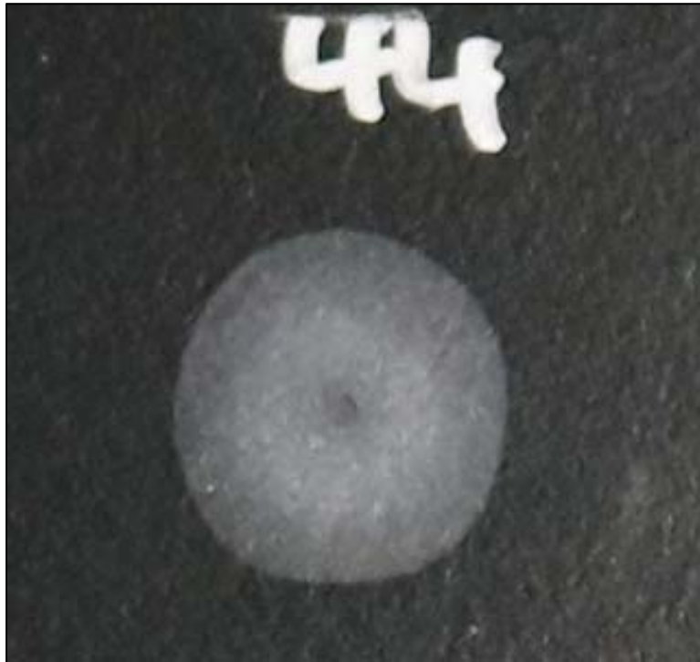
Chemical spot test #44, Sulfuric Acid (96%), Rating 2, Gloss change
